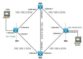
Fig 1. The Virtual High-Speed Network Laboratory Reference Topology
